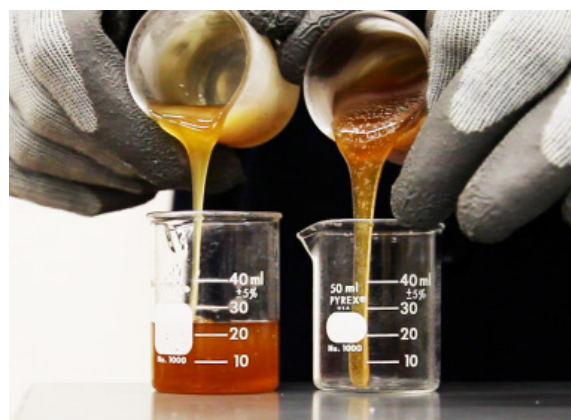
HyFilm LEO HDEO 5W-30 Flow vs. 15W-40 at -35° C. Time elapsed 50 seconds.
